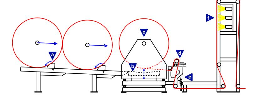
Shown above is a drawing that better illustrates the operation of the shaftless unwind stand with a back-lighted oprator inspection tower (also shown on top of opposite page). Use the key below for more information:
