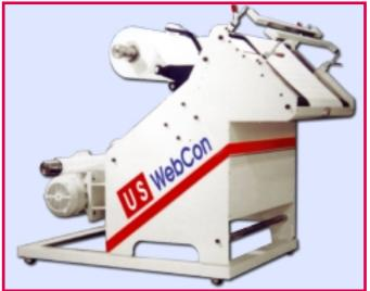
This unit, The Mutt, is an inspection winder with slitting capability. It has been designed to allow an operator to inspect the web and perform any splicing operations necessary from the workstation. The unit will accept score, shear, or razor slitting, and it can be supplied with a center driven simplex or duplex winding station. The Mutt is fully cantilevered and is supplied with tension control and edge guiding.
